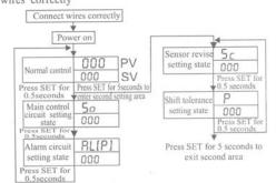
B: Specialist type PID, specialist type PID + alarm etc. instrument' operation flow:
